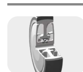
Construction of wheel: ball bearing, sealed
