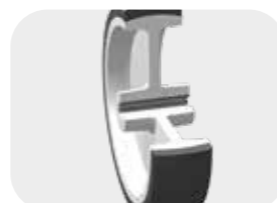
section view wheel with plain bearing
